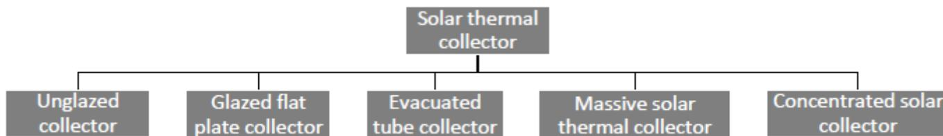
Types of solar thermal collectors
